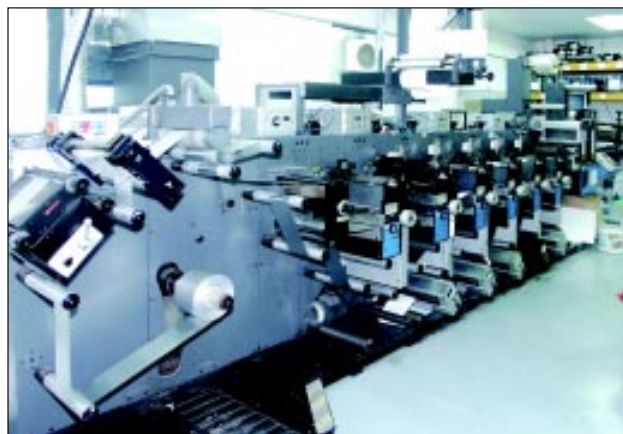
The six colour narrow band web flexo press prints high quality adhesive labels
